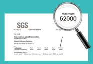
Accugrip's gloves coating didn't break until 52,000 cycles in EN388
